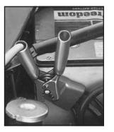
Don't let the other end touch metal. Connect it to the positive (+) terminal of the good battery. Use a remote positive (+) terminal if the vehicle has one.
